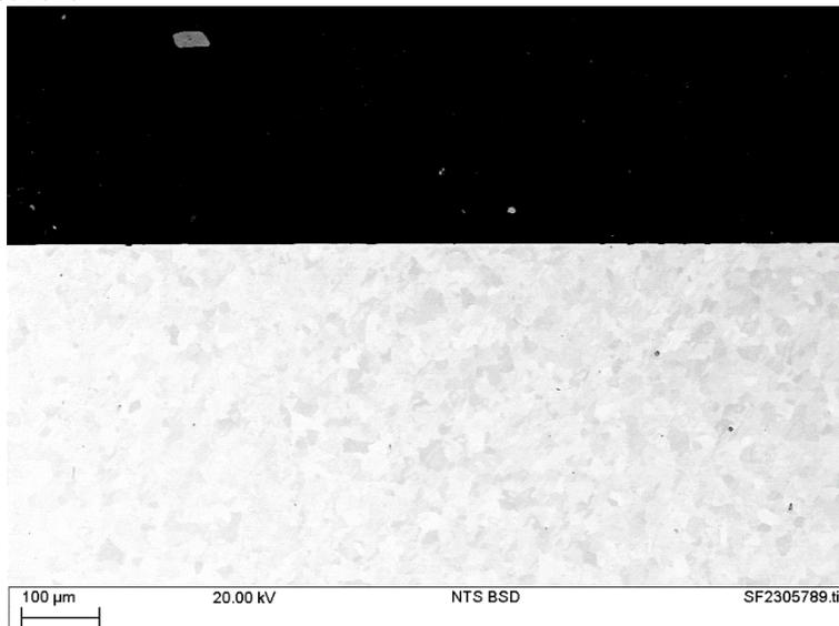
**Figure 8 SEM image of a cross-section of sample SA105-600-4 following exposure testing.**
