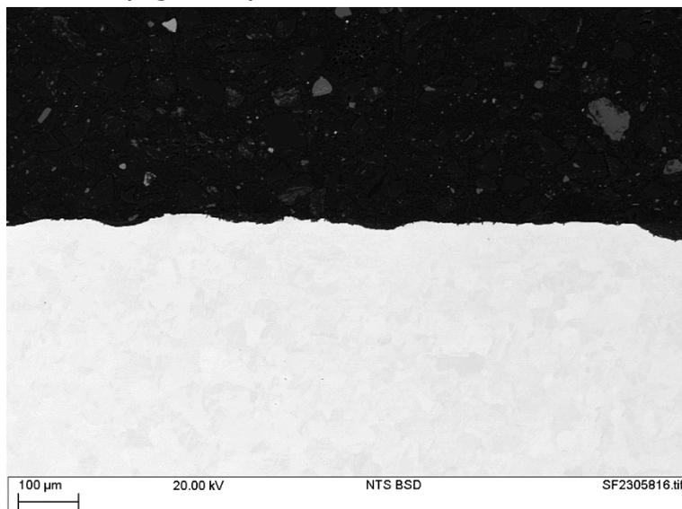
Figure 14 SEM image of a cross-section of sample 304L-AR-5 following exposure testing.
