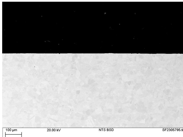
Figure 20 SEM image of a cross-section of sample 316L-600-5 following exposure testing.
