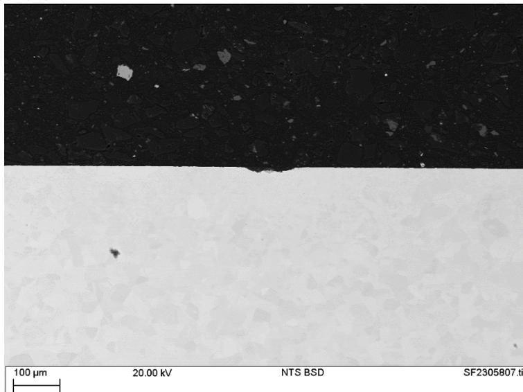
Figure 16 SEM image of a cross-section of sample 304L-600-5 following exposure testing.
