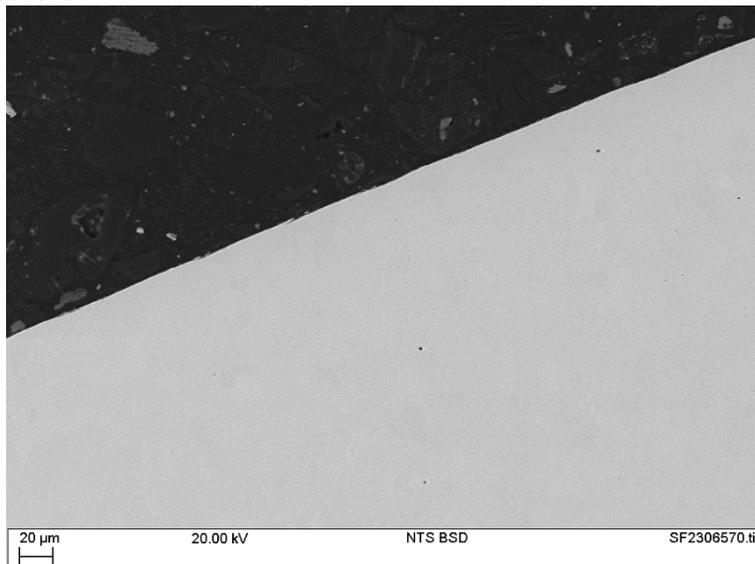
Figure 12 SEM image of a cross-section of sample SA179-600-3 following exposure testing.
