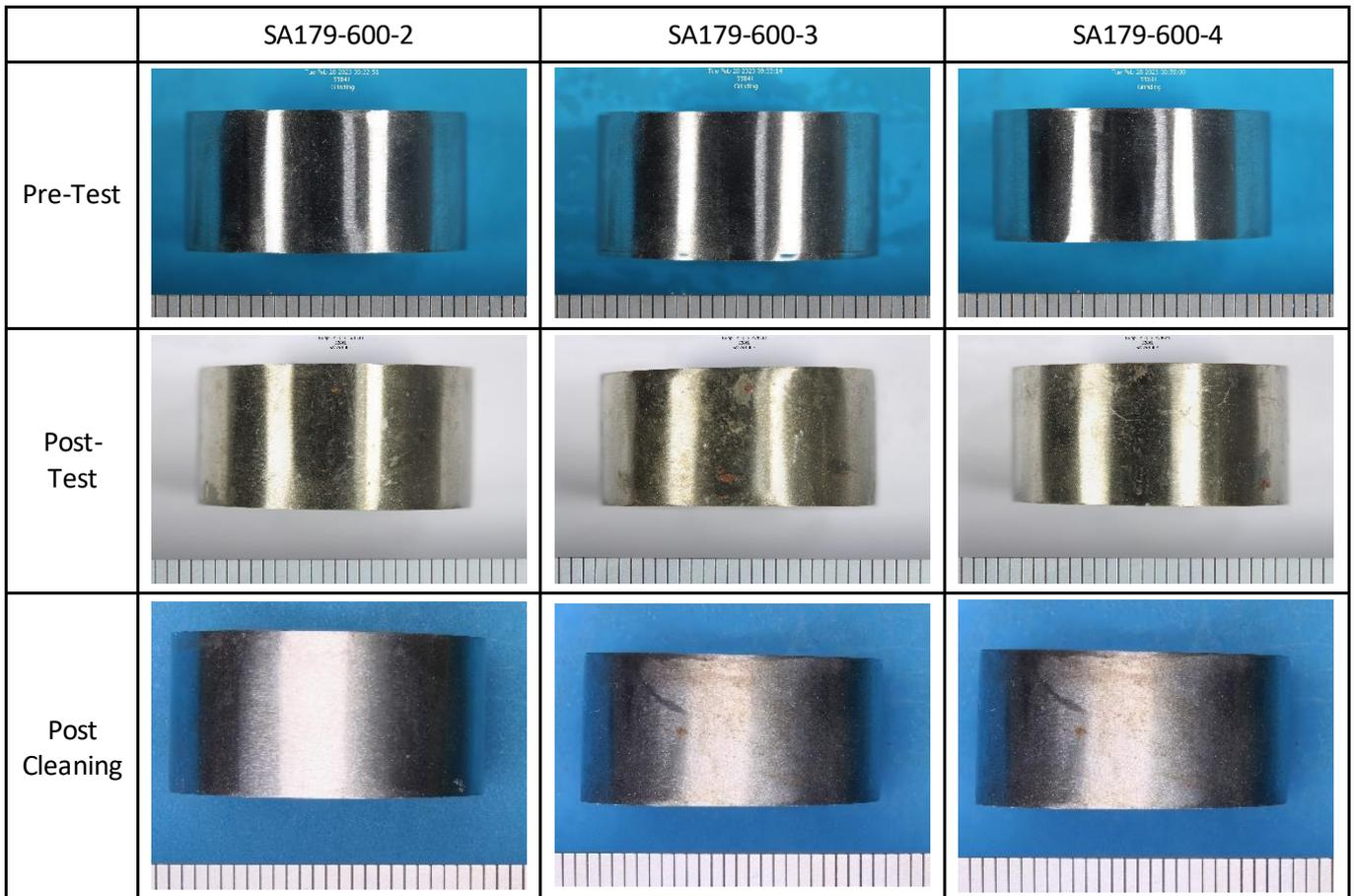
Figure 11 Photographs showing samples composed of SA179 prepared to a 600 grit finish before testing, after testing and post-cleaning.
