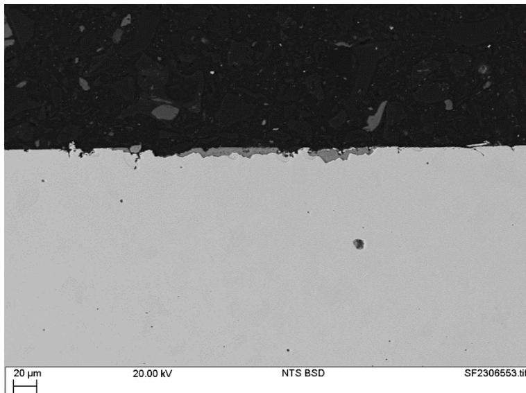
Figure 10 SEM image of a cross-section of sample SA179-AR-1 following exposure testing.
