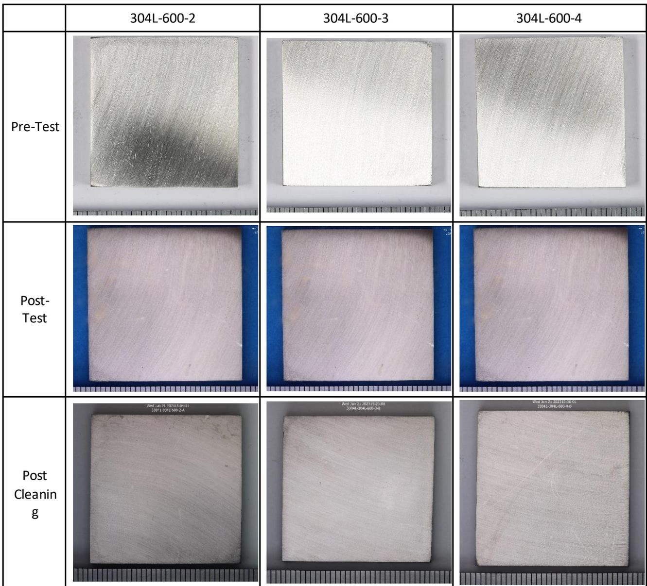
**Figure 15** Photographs showing samples composed of 304L prepared to a 600 grit finish before testing, after testing and post-cleaning.
