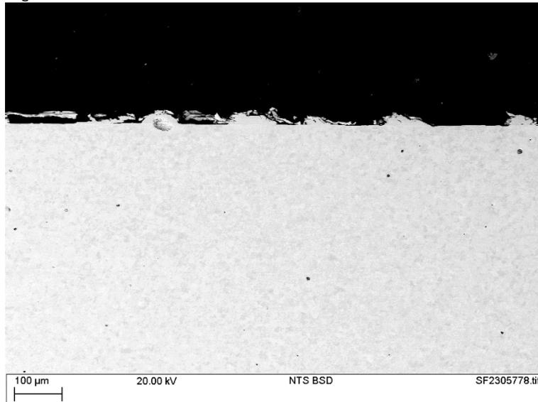
**Figure 4 SEM image of a cross-section of sample SA516-600-4 following exposure testing.**
