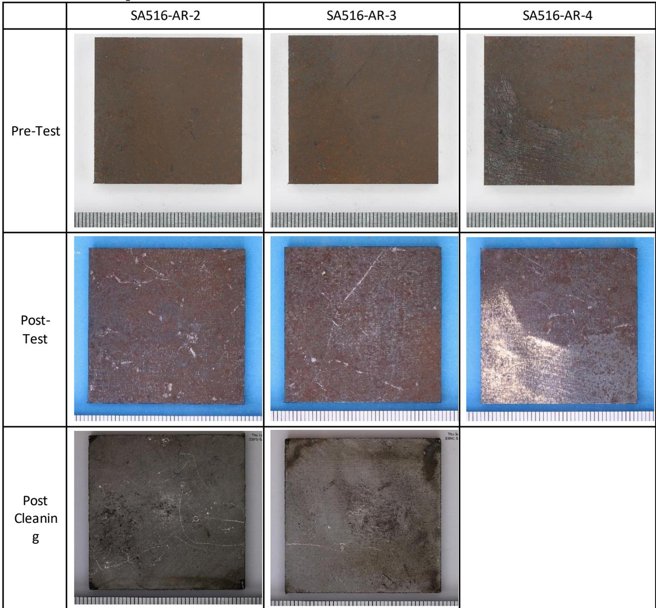
Figure 1 Photographs showing samples composed of SA516 in the as-received condition before testing, after testing and post-cleaning.
