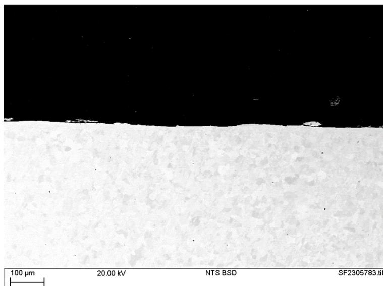
Figure 6 SEM image of a cross-section of sample SA105-AR-5 following exposure testing.
