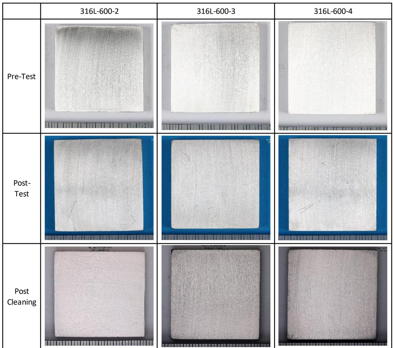
Figure 19 Photographs showing samples composed of 316L prepared to a 600 grit finish before testing, after testing and post-cleaning.
