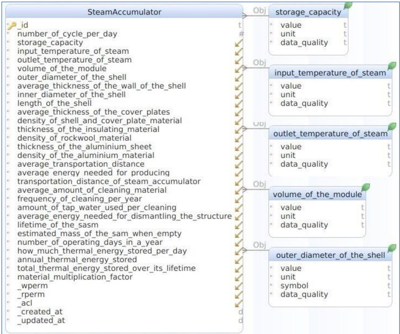
Figure A6 ER diagram of steam accumulator table
