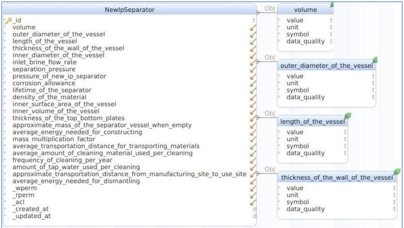
Figure A1 ER diagram of new IP separator table
