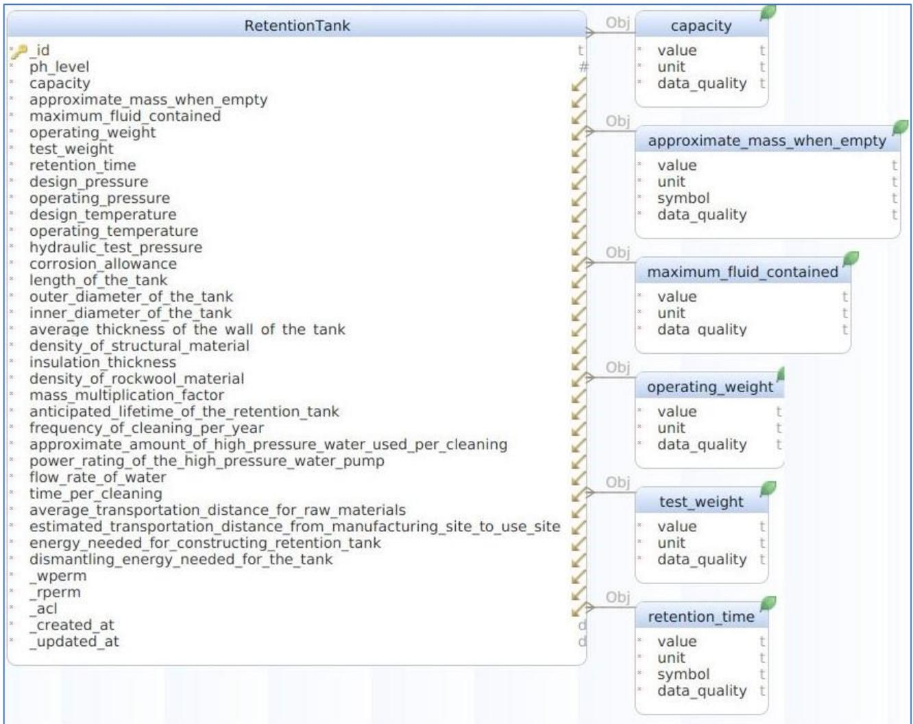
Figure A3 ER diagram of retention tank table
