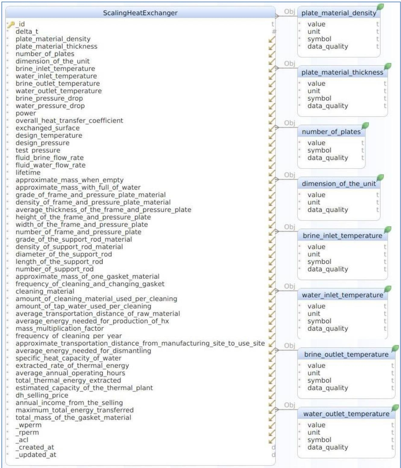
Figure A4 ER diagram of scaling heat exchanger table
